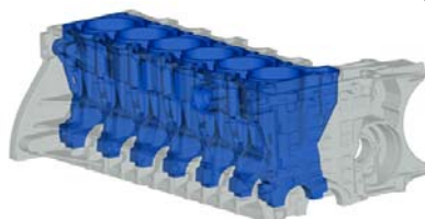
BMW Block with Cast in Al-Si Liners
